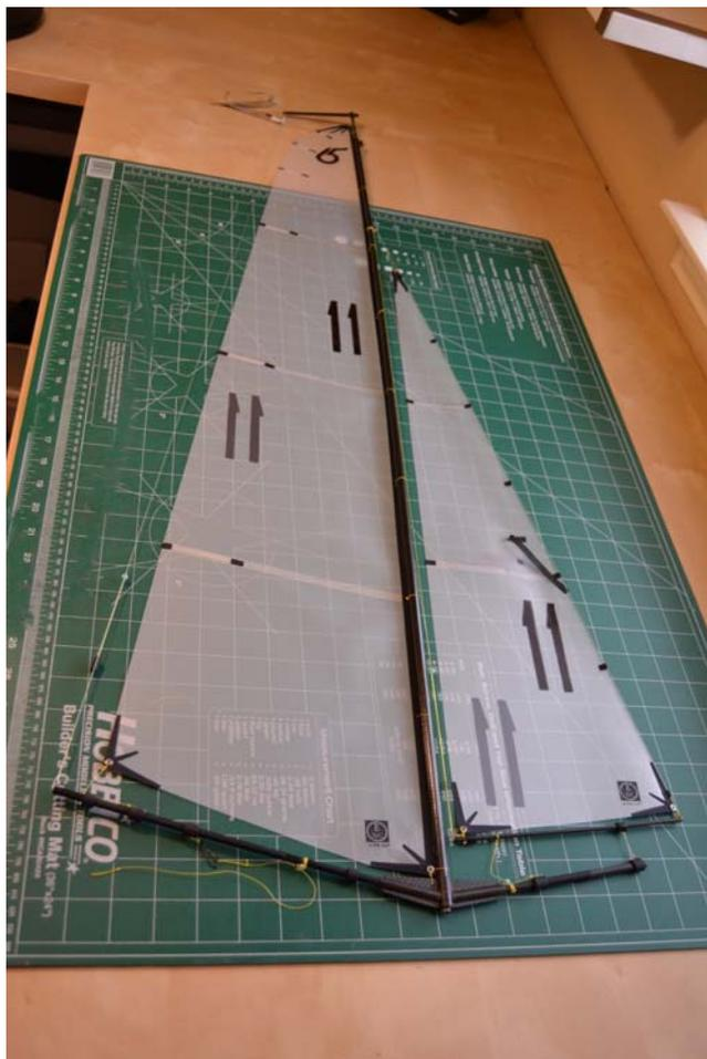
At right is a picture the main boom. The tack is attached to a line that goes through a hole in the T fitting and back to the first black neoprene tube. You adjust the tension on the downhaul by moving this tube back and forth. Other than bowsies on the topping lifts, forestay, and jib halyard, all other adjustments are made by moving the various tube segments on the booms.
