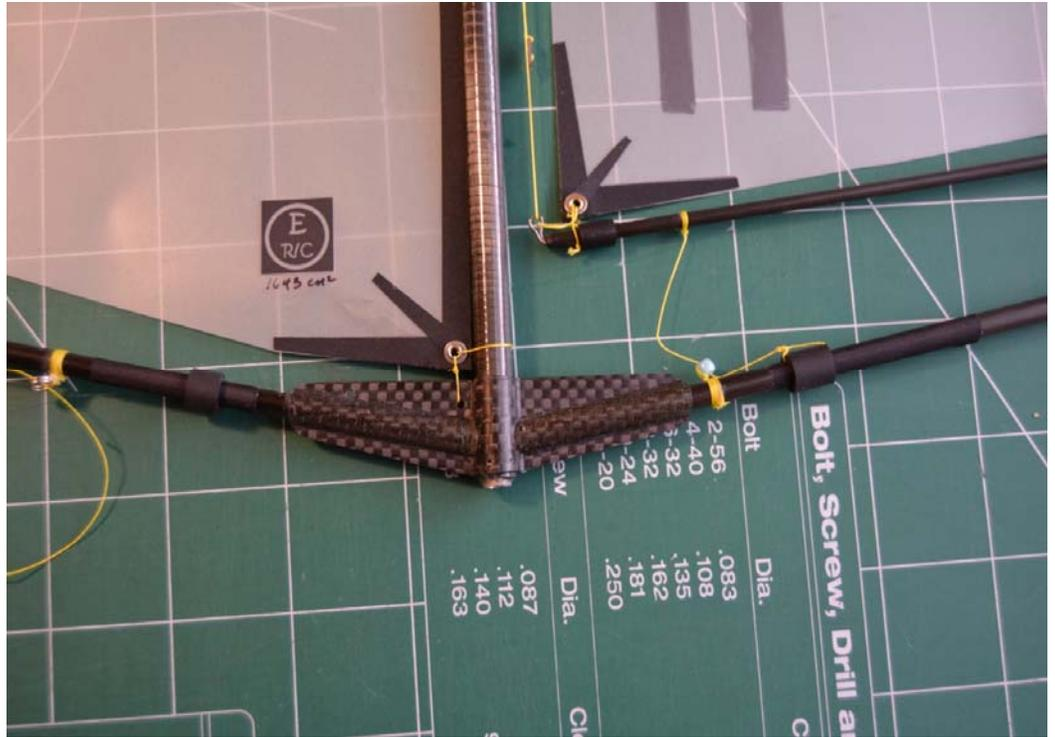
The jib boom pivots on the short connector line at the front of the forward spar. The boom can be moved forward to change the balance of the rig.
