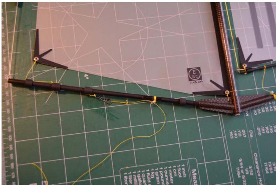
At the back of the boom is a cotter pin, and this is the turn point for the backstay of the rig. The backstay should always have enough tension so that the sail leech is not loaded up. If you release the backstay and store the sails, the panels will slowly pull apart.
