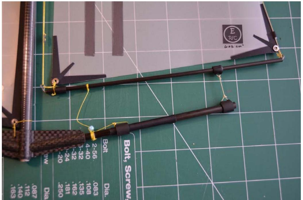
The crane is a molded CF part, but a bent wire will work just fine. The wire needs to be relatively stiff, so something about 1/16" in diameter is about right.
